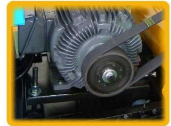
槓桿式皮帶調整結構 Easy maintenance mechanism
